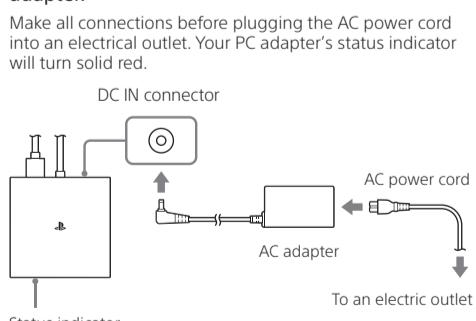
Make all connections before plugging the AC power cord into an electrical outlet. Your PC adapter's status indicator will turn solid red.
