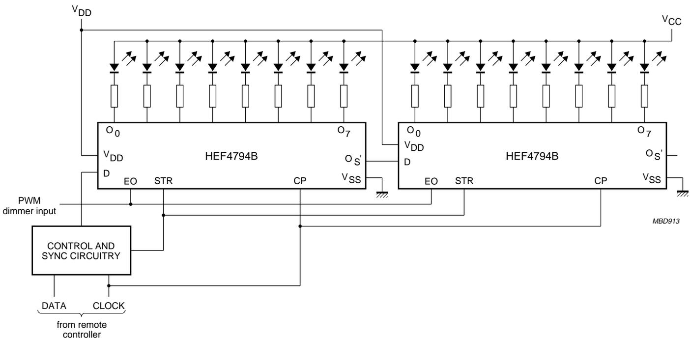
Fig.6 Application example: serial-to-parallel converting LED drivers.
