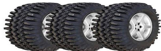
Fig4: Cross ply Tyre
